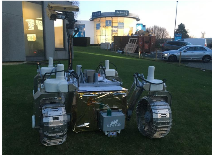
FIGURE 3. NEWTON instrument integrated into LUVMI rover platform (LUVMI H2020 project, Grant Agreement: 727220).
