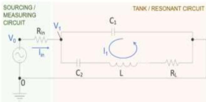
Figure 2.- Modified tank circuit scheme.
